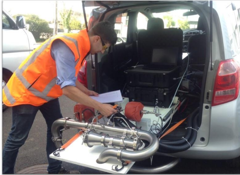
Figure 4: PEMS equipment being installed in a test vehicle in Auckland
