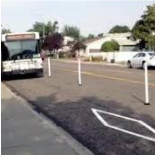
Figure 3C. A separated lane with posts (also known as bollards)
