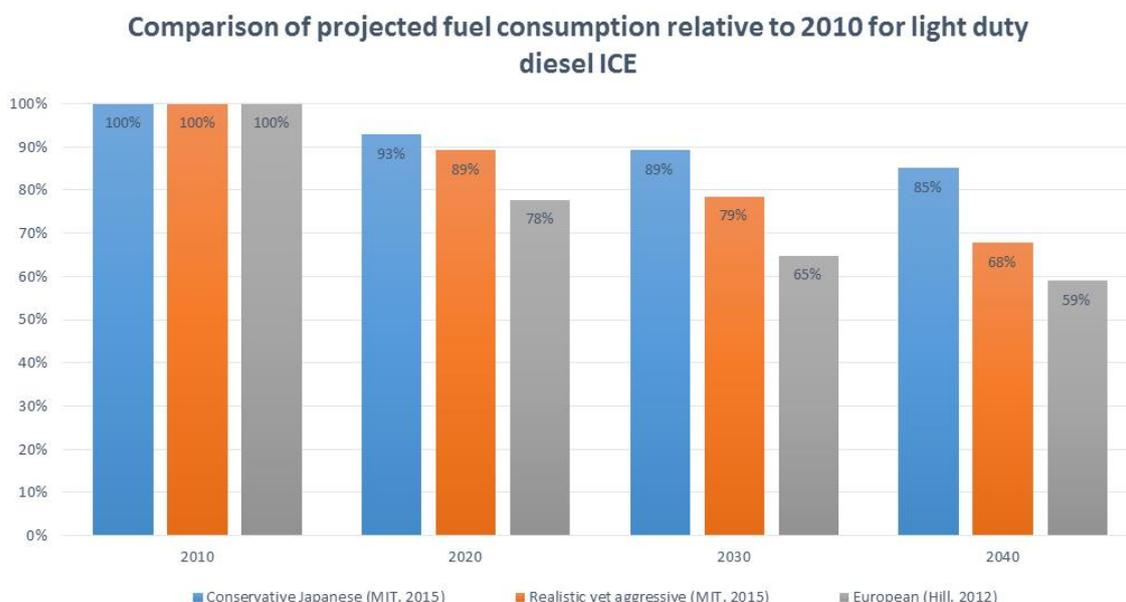
**Figure 7:** Comparison of projected fuel consumption relative to 2010 for light duty diesel ICE
