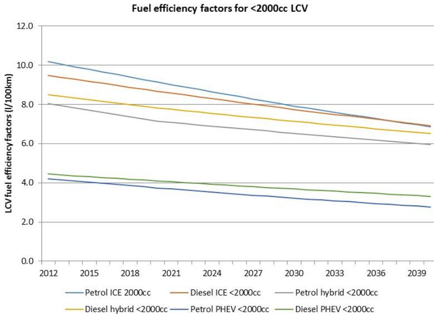
**Figure 11:** Fuel efficiency factors and projections for LCV <2000cc
