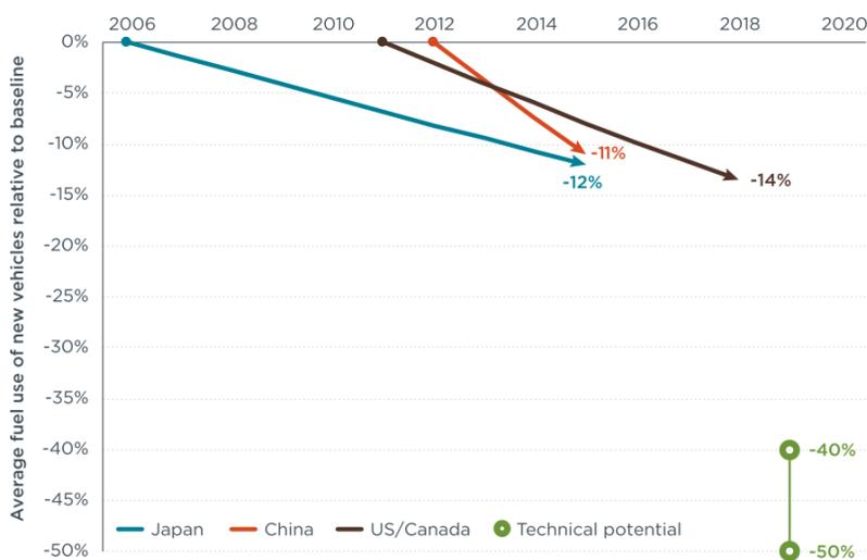
**Figure 9.** Global comparison of heavy-duty vehicle efficiency standards
