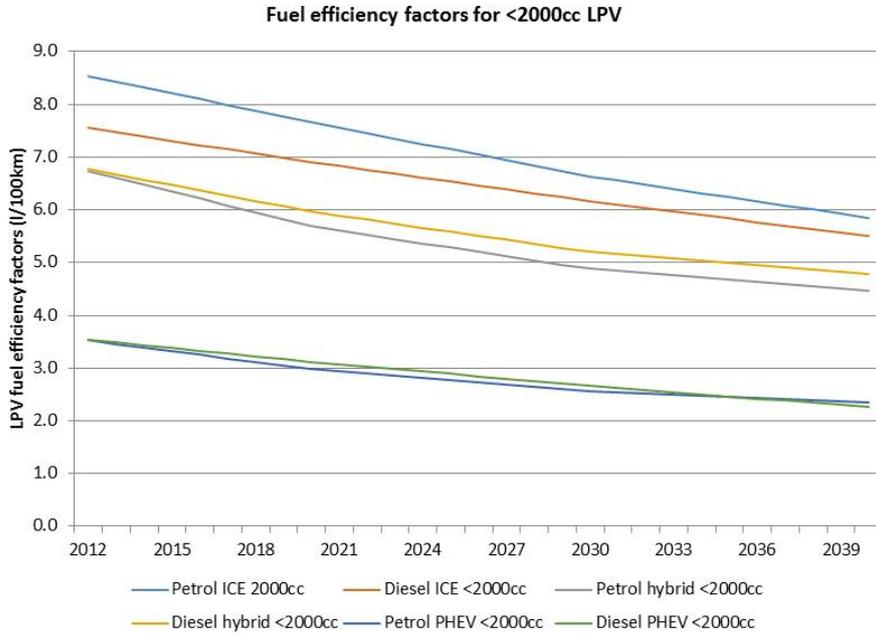
**Figure 10:** Fuel efficiency factors and projections for LPV <2000cc
