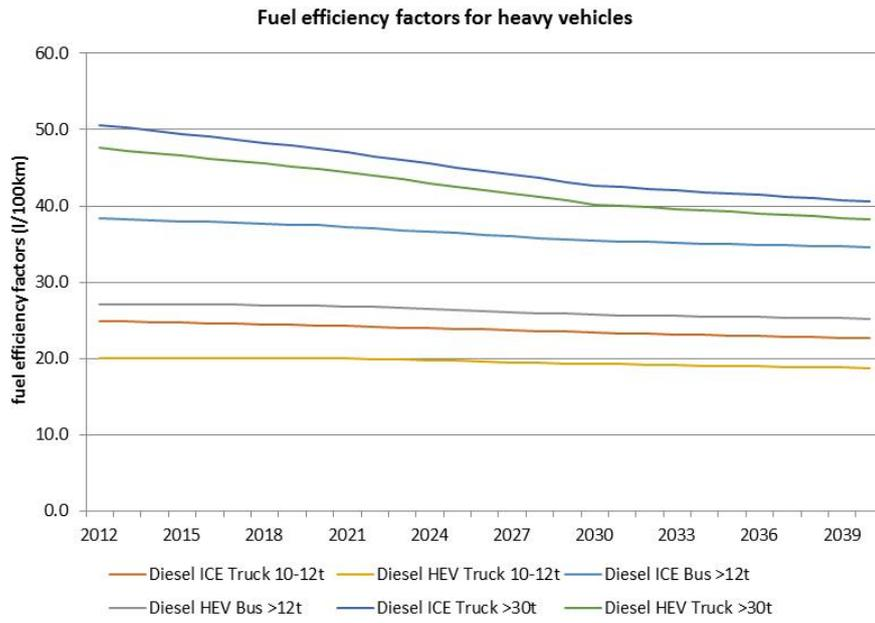
**Figure 12:** Fuel efficiency factors and projections for heavy vehicles
