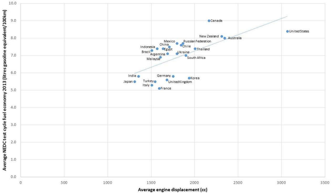
**Figure 3:** Comparison of average fuel economy (l/100km) and engine displacement (cc) for light duty vehicles internationally [Source: OECD/IEA 2016 and MoT. See accompanying spreadsheet for details]
