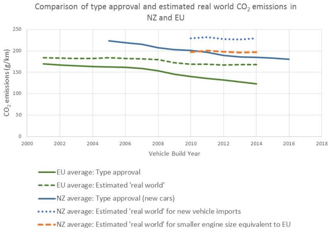
**Figure 5:** Comparison of type approval and estimated real world CO<sub>2</sub> emissions in New Zealand and Europe [Source: ICCT, 2015b and MoT, 2016. See accompanying spreadsheet for details]
