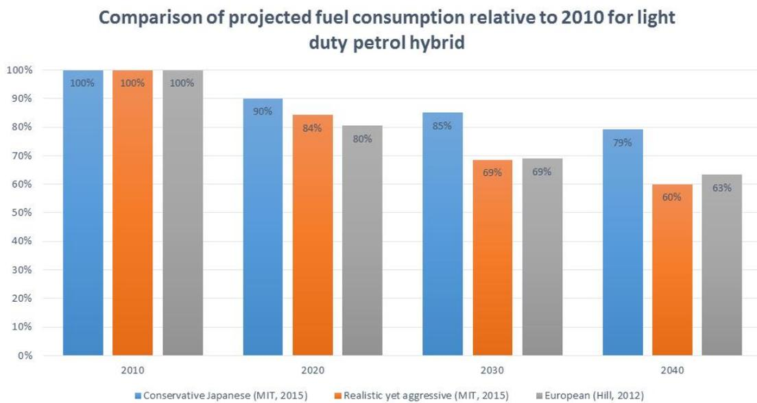
**Figure 8:** Comparison of projected fuel consumption relative to 2010 for light duty petrol hybrid
