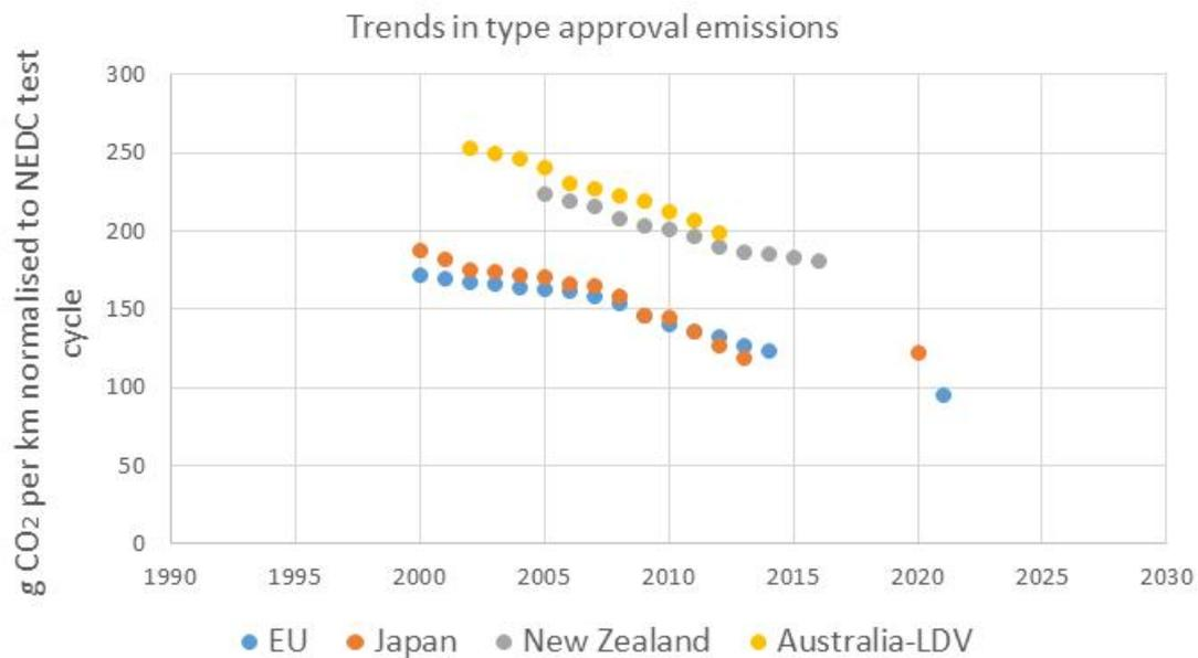
**Figure 2:** Trends in average type approval CO<sub>2</sub> emissions from new vehicles in New Zealand compared with Europe, Japan and Australia [Source: ICCT, 2015b and MoT, 2016. See accompanying spreadsheet for details]
