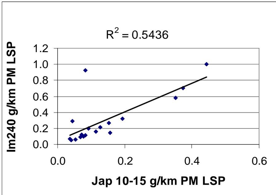
Figure 36: IM240 PM (g/km) LLSP Versus Jap10-15 PM (g/km) LSP for EFRU Light Vehicle Tests.
