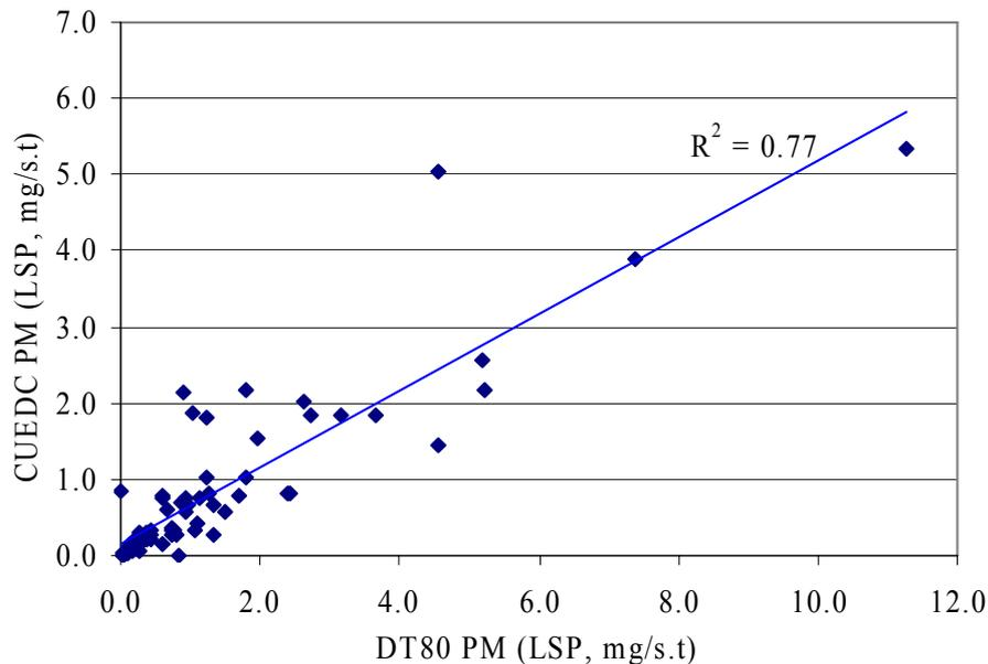
**Figure 20: CUEDC PM (mg/s.t) versus DT80 PM (mg/s.t) for Light and Heavy Vehicles Tested in Australia.**
