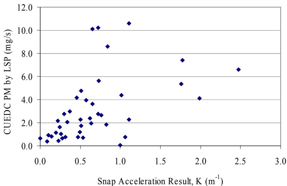
**Figure 16: CUEDC PM Versus Snap Acceleration Result for Heavy Vehicles Tested in Australia.**
