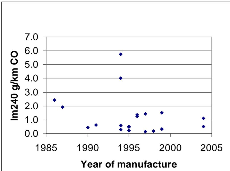
Figure 54: IM240 CO g/km Versus Year of Manufacture for EFRU Light Vehicle Tests.
