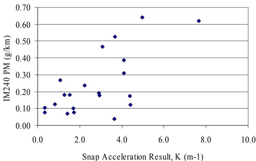
**Figure 14: IM240 PM Versus Snap Acceleration Result for Light Diesel Vehicles Subject to Detailed Dynamometer Testing at the EFRU Laboratory.**
