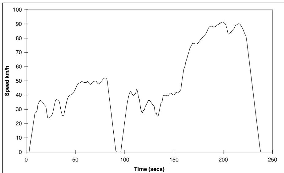
**Figure 32: Vehicle Speed During the IM240 Drive Cycle.**
