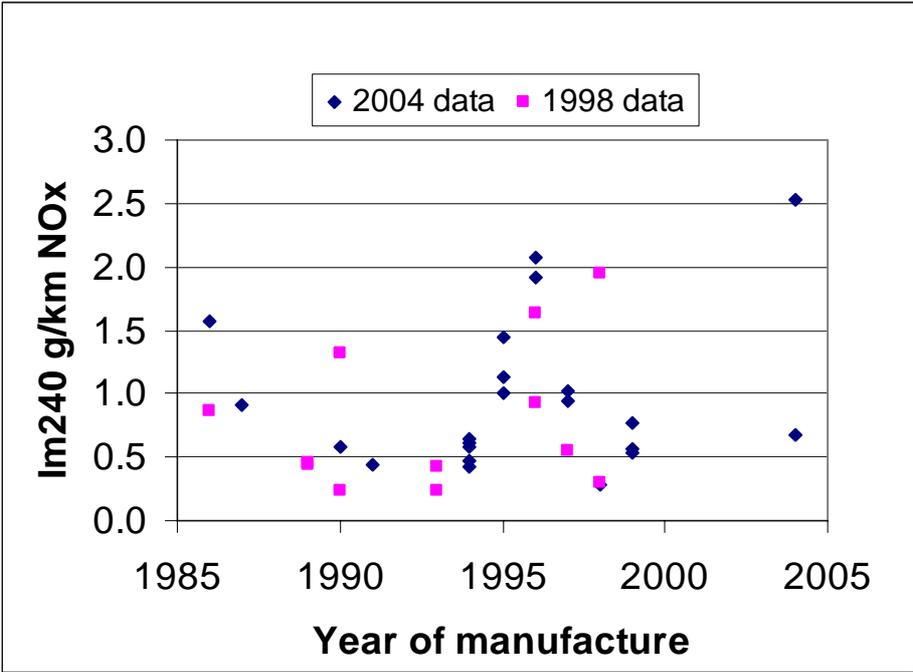
Figure 55: IM240 NOx g/km Versus Year of Manufacture for EFRU Light Vehicle Tests.
