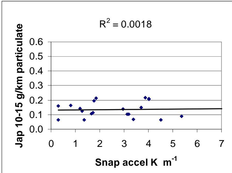
Figure 47: Jap10-15 PM (g/km) Versus Snap acceleration K for EFRU Light Vehicle Tests.
