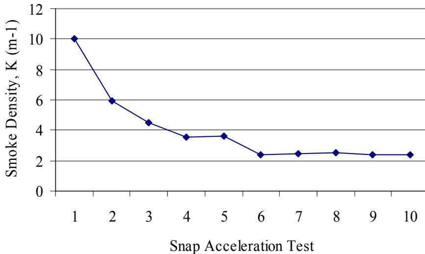
**Figure 4: Consecutive Individual Acceleration Results for a Light Diesel Vehicle (Reg. No. RQ3666) Exhibiting Lowered Results with First Accelerations.**
