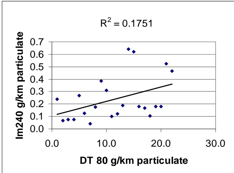
Figure 39: IM240 PM (g/km) Versus DT80 PM (g/km) for EFRU Light Vehicle Tests.
