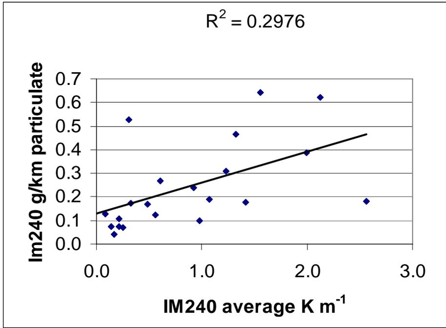
Figure 57: IM240 PM g/km Versus IM240 average K for EFRU Light Vehicle Tests.
