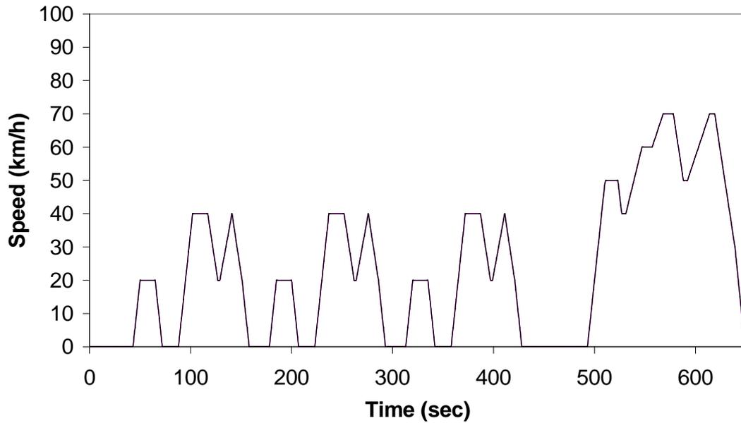
**Figure 31: Vehicle Speed During the Jap10-15 Drive Cycle.**
