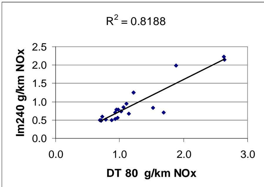
**Figure 42: IM240 NOx (g/km) Versus DT80 NOx (g/km) for EFRU Light Vehicle Tests.**
