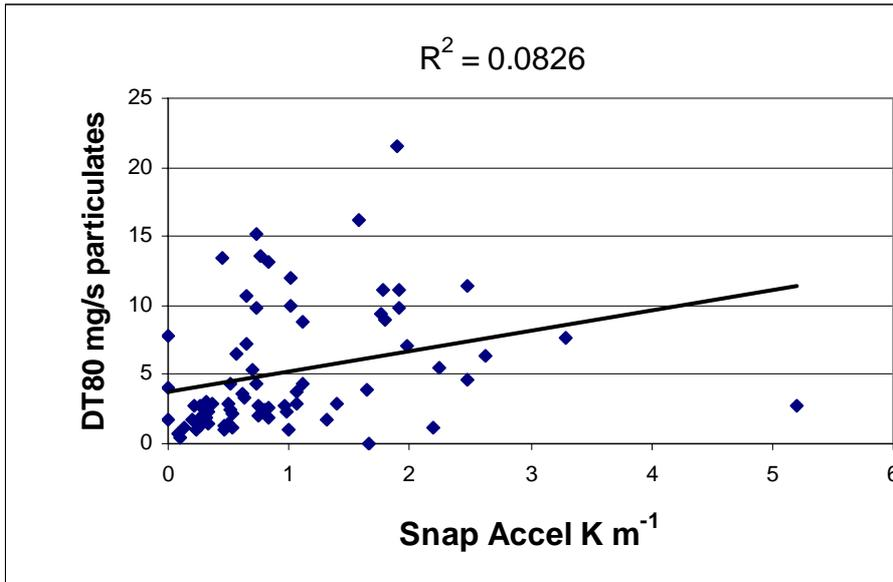
**Figure 63: Australian DT 80 PM (g/s) (DustTraK) Versus Snap Acceleration K (m -1) for all Classes of Diesel Vehicles.**
