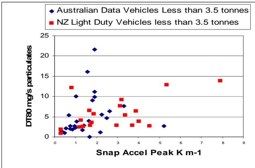
**Figure 64: DT 80 PM (g/s) (DustTraK) Versus Snap Acceleration K (m -1) for Australian MC and NA Class Diesel Vehicles and all New Zealand Light Diesel Vehicles.**
