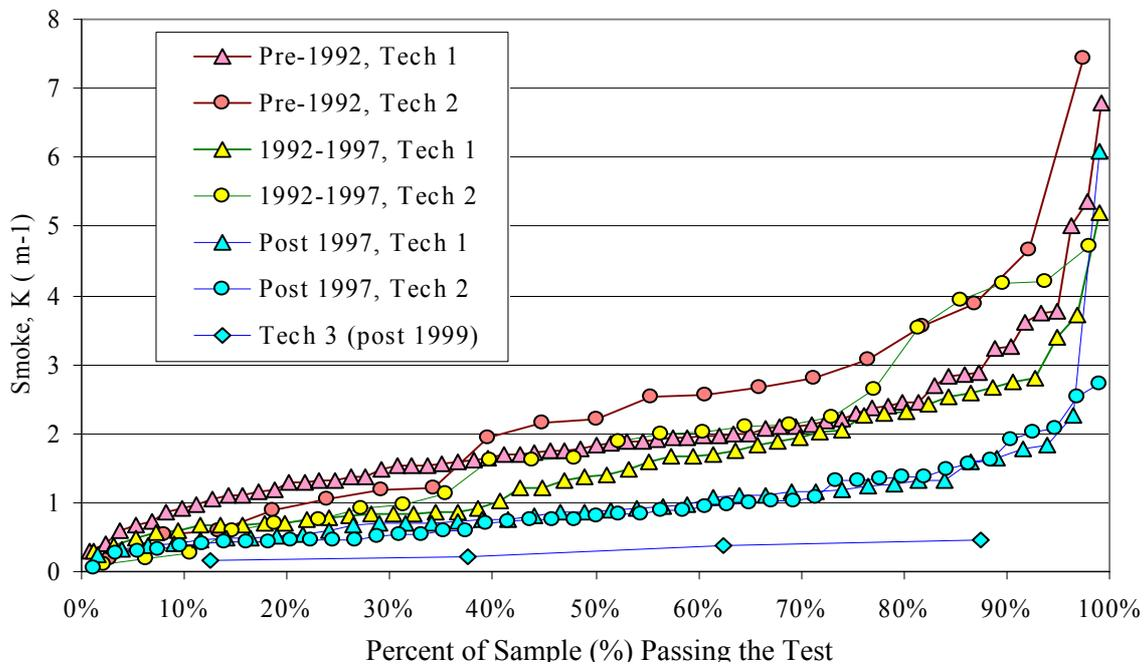
**Figure 12: Percentile Plots for the Profiling Snap Acceleration Data Set for Heavy Diesel Vehicles Divided by Technology and YoM Groups.**
