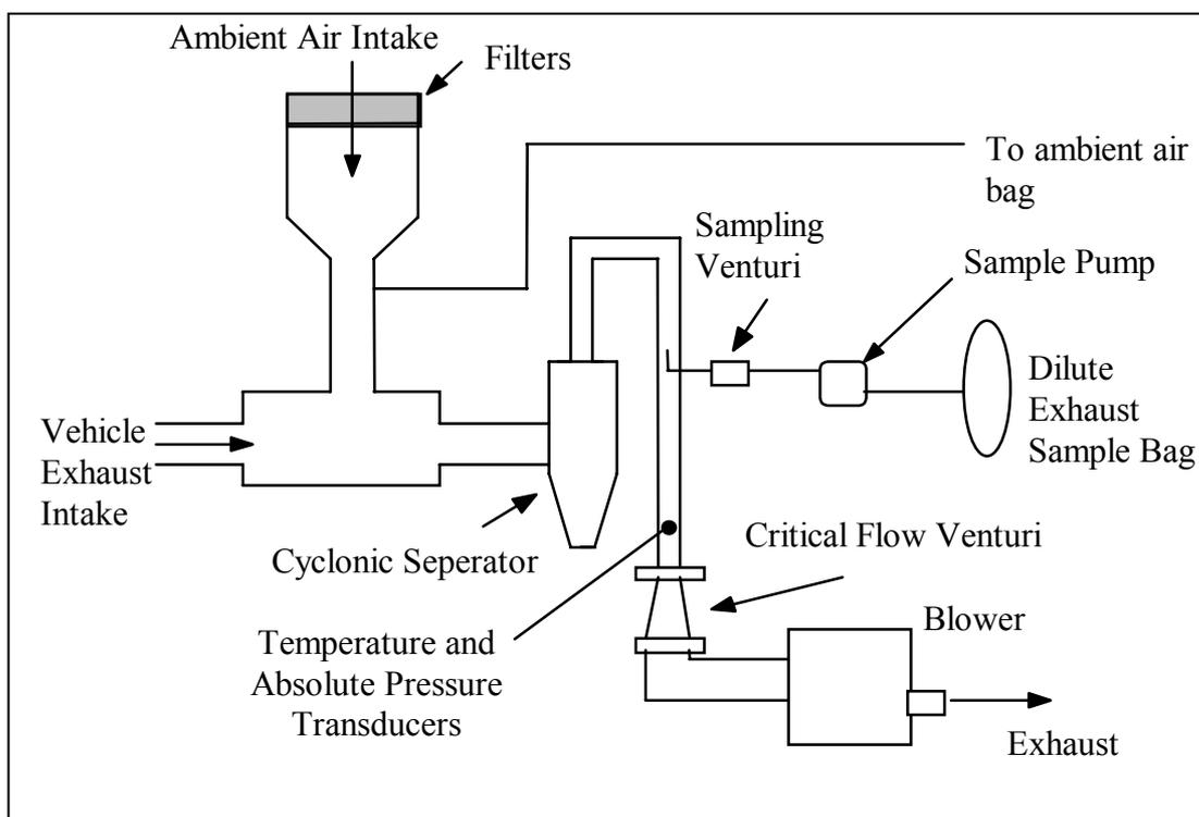
**Figure 29: Schematic of the CVS System.**
