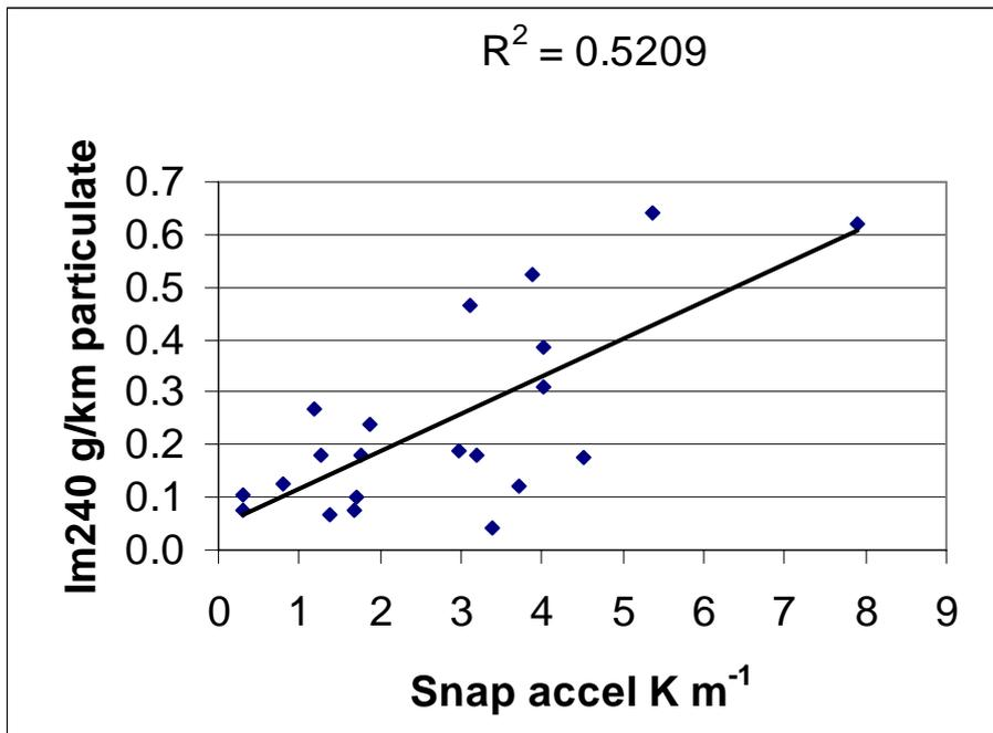
Figure 46: IM240 PM (g/km) Versus Snap Acceleration  $K m^{-1}$  for EFRU Light Vehicle Tests.
