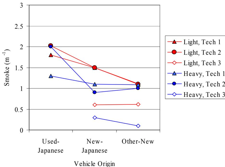
**Figure 10: Median Snap Acceleration Results (Smoke Density,  $K m^{-1}$ ) for Light and Heavy Diesel Vehicles by Technology and Origin for the Adjusted Snap Acceleration Data Set.**
