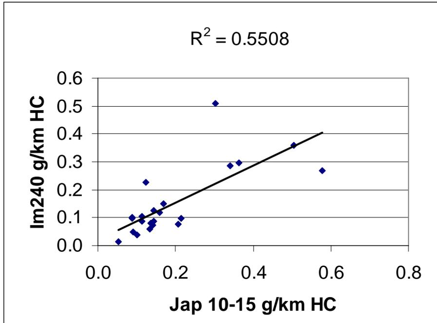
Figure 37: IM240 HC (g/km) Versus Jap10-15 HC (g/km) for EFRU Light Vehicle Tests.
