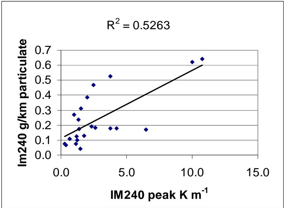
Figure 56: IM240 PM g/km Versus IM240 peak K for EFRU Light Vehicle Tests.
