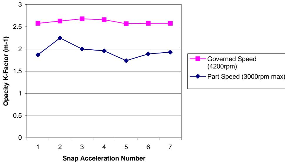
**Figure 25: Successive Snap Acceleration Results for a Mitsubishi Canter Tested with the Accelerator Released After Reaching High Governed Speed and After Reaching a Lesser Engine Speed.**
