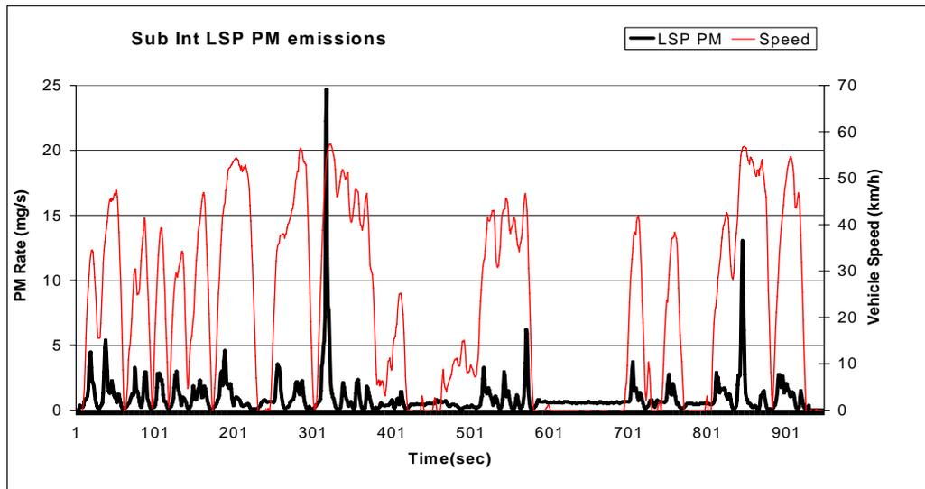
**Figure 18: LSP Emissions Measured over the Suburban Interrupted Driving Schedule for a Nissan Laurel (results from a 2001 BP test programme using low-sulphur diesel for the vehicle in as-received condition).**
