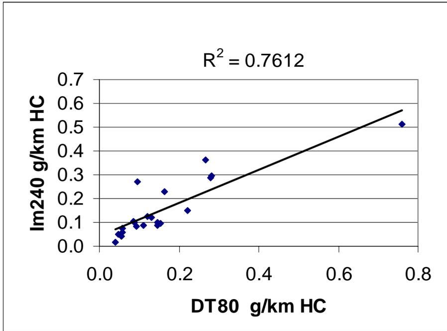
**Figure 41: IM240 HC (g/km) Versus DT80 HC (g/km) for EFRU Light Vehicle Tests.**
