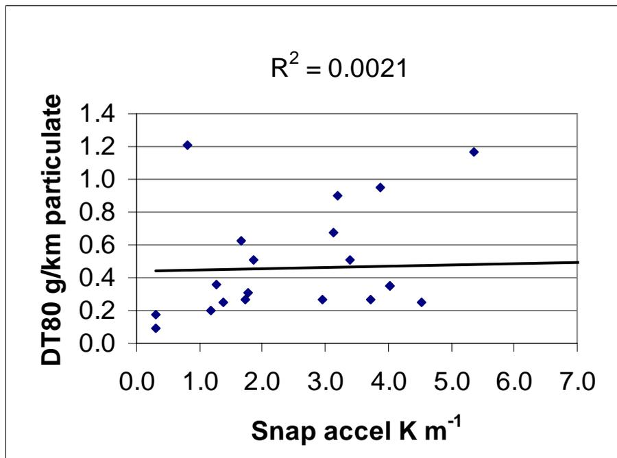
Figure 48: DT80 PM (g/km) Versus Snap Acceleration K for EFRU Light Vehicle Tests.
