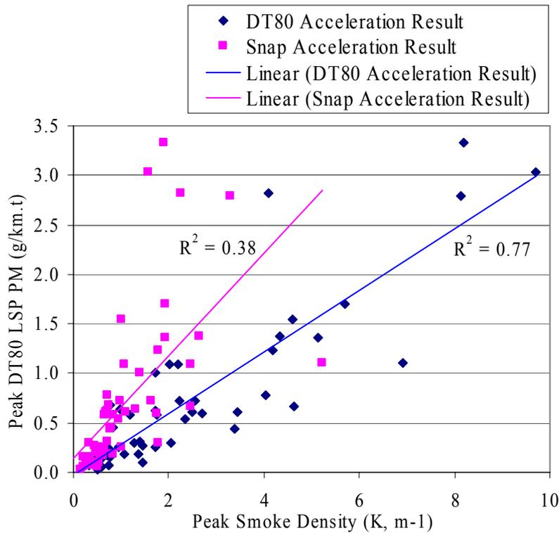
**Figure 19: Peak DT80 PM (LSP) Versus Peak Smoke Density Measured During That DT80 Test and During a Snap Acceleration Test of Same Vehicles.**
