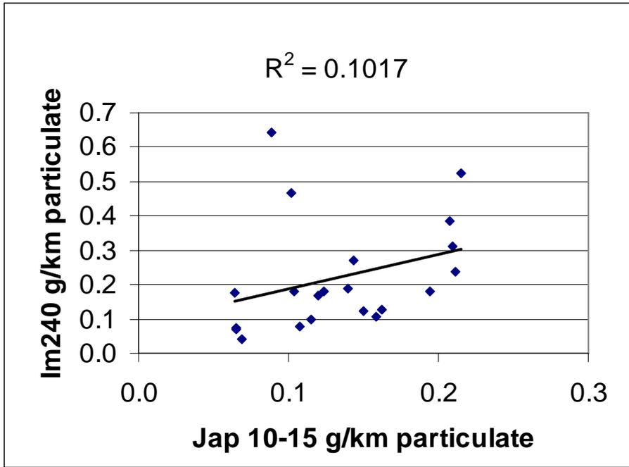
Figure 35: IM240 PM (g/km) Versus Jap10-15 PM (g/km) for EFRU Light Vehicle Tests.
