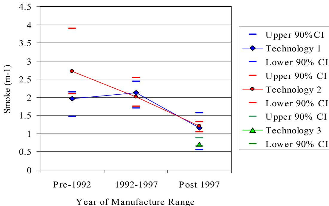
**Figure 27: Median Snap Acceleration Results (Smoke Density, K, m<sup>-1</sup>) for Light Diesel Vehicles by Technology and YoM Range for the Adjusted Snap Acceleration Data Set.**
