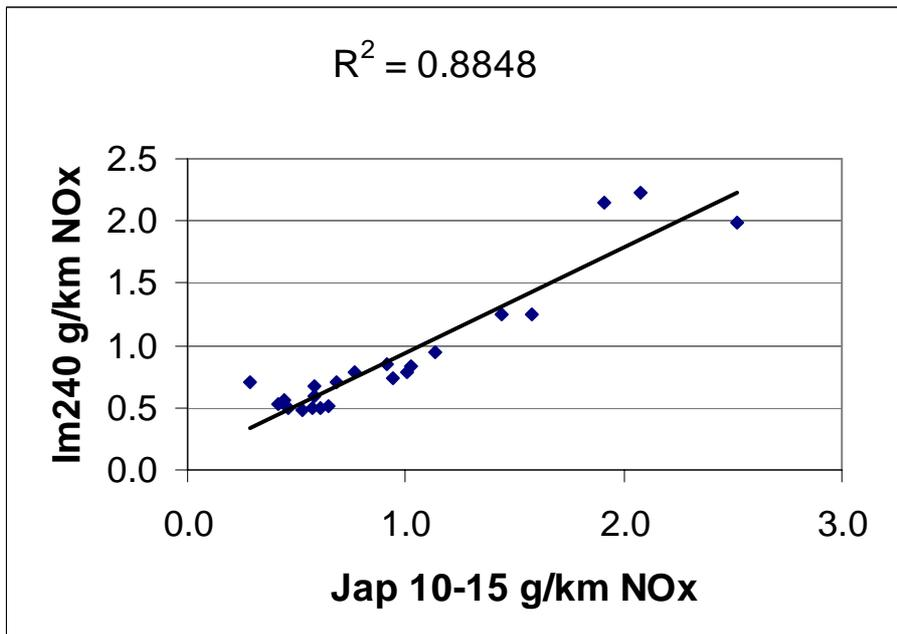
Figure 38: IM240 NOx (g/km) Versus Jap10-15 NOx (g/km) for EFRU Light Vehicle Tests.
