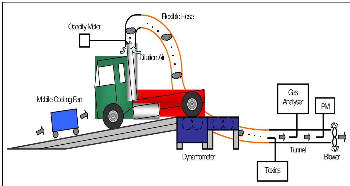
**Figure 34: Schematic of the Diesel Test Australia Chassis Dynamometer Test Arrangement**
