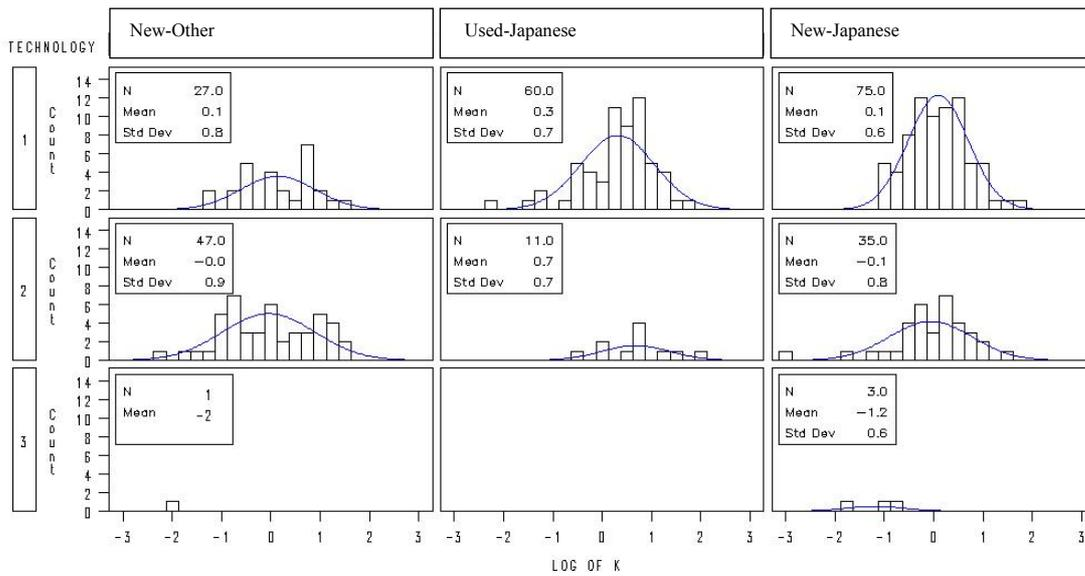
**Figure 9: Log K for the Adjusted Snap Acceleration Sample of Light Diesel Vehicles Divided by Technology and Origin.**
