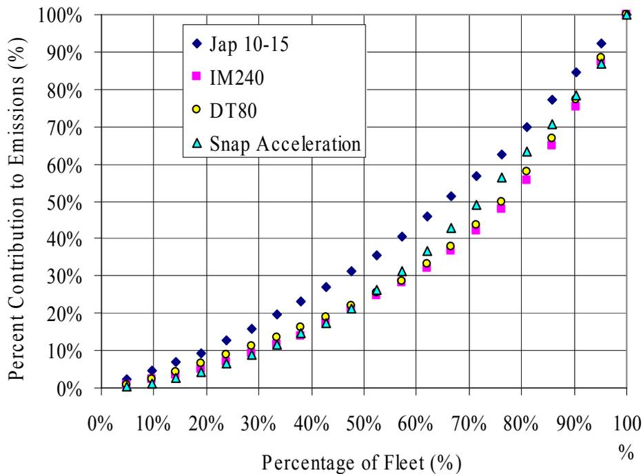
**Figure 15: Cumulative PM Emissions by the Jap 10-15, IM240 and DT80 Test Procedures and Pilot's Snap Acceleration Procedure for the Light Diesel Vehicles Subject to Dynamometer Testing at the EFRU Laboratory.**
