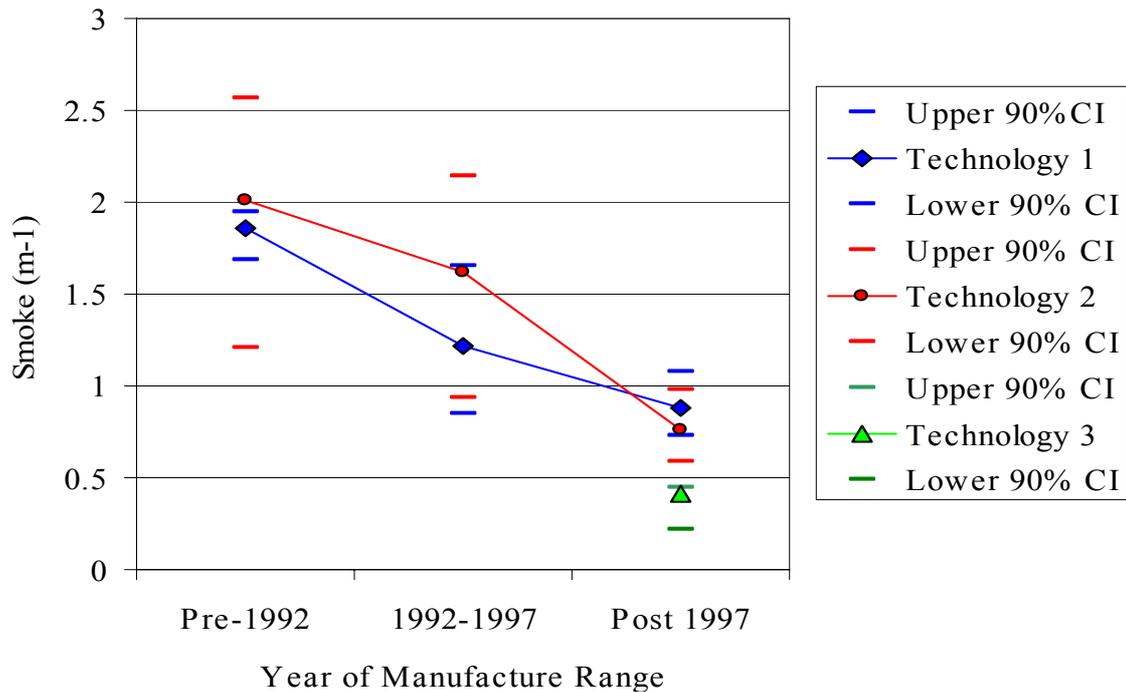
**Figure 28: Median Snap Acceleration Results (Smoke Density,  $K, m^{-1}$ ) for Heavy Diesel Vehicles by Technology and YoM Range for the Adjusted Snap Acceleration Data Set.**
