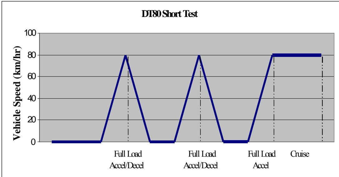
**Figure 33: Vehicle Speed During the DT80 Test Procedure.**
