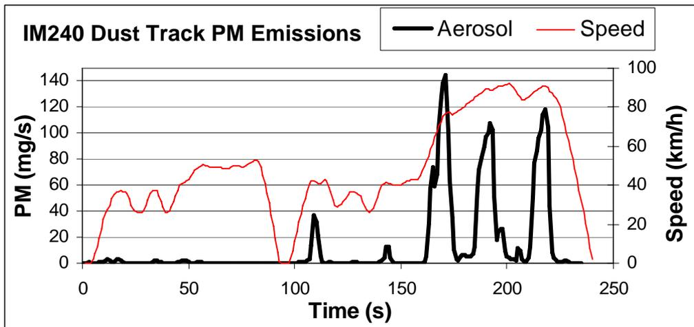
**Figure 21: Real Time PM, as Measured by Light Scattering Photometer over the IM240 Test Cycle, for a Light Diesel Vehicle in Poor Condition (the Toyota Estima in As-Received Condition).**
