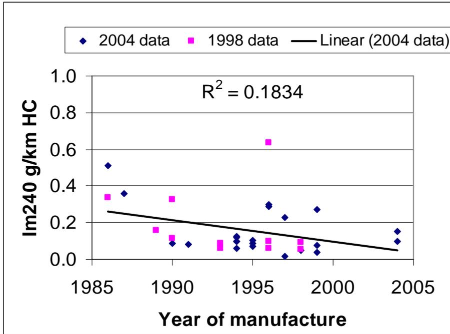
Figure 53: IM240 HC g/km Versus Year of Manufacture for EFRU Light Vehicle Tests.
