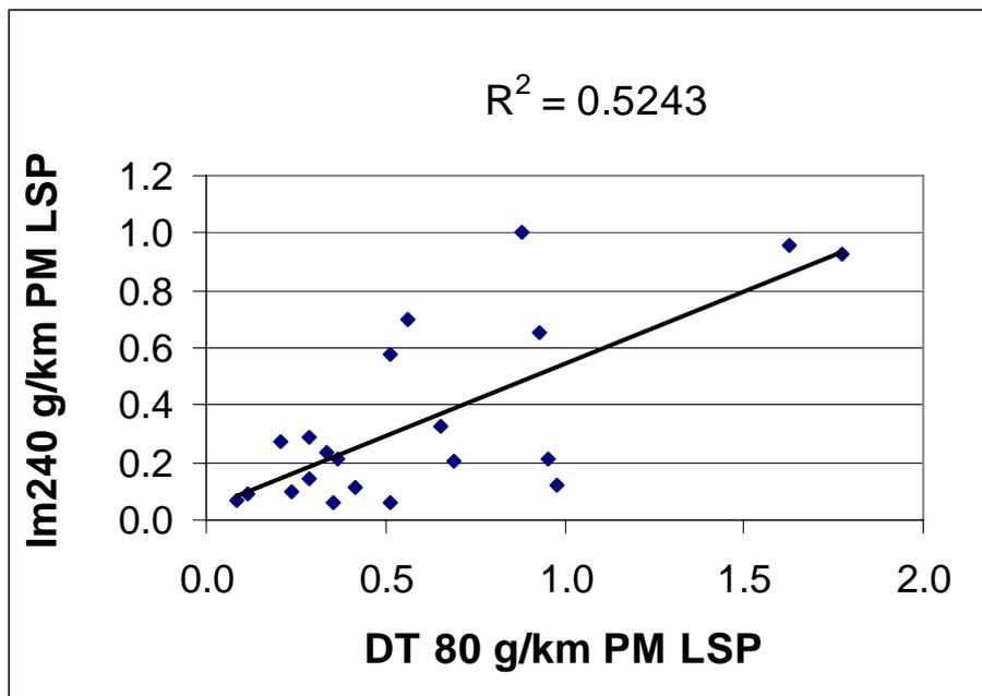
Figure 40: IM240 PM (g/km) LSP Versus DT80 PM (g/km) LSP for EFRU Light Vehicle Tests.
