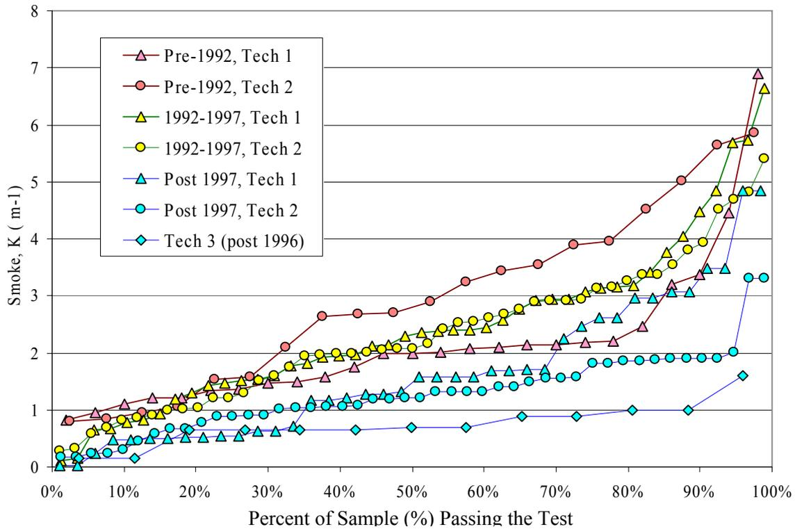
**Figure 11: Percentile Plots for the Profiling Snap Acceleration Data Set for Light Diesel Vehicles Divided by Technology and YoM Groups.**
