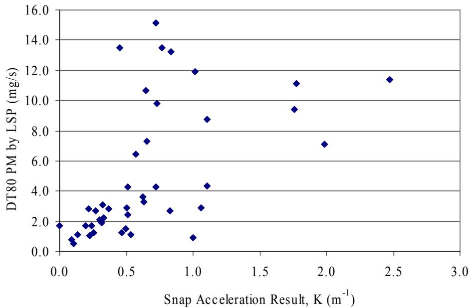
**Figure 17: DT80 PM Versus Snap Acceleration Result for Heavy Vehicles Tested in Australia.**
