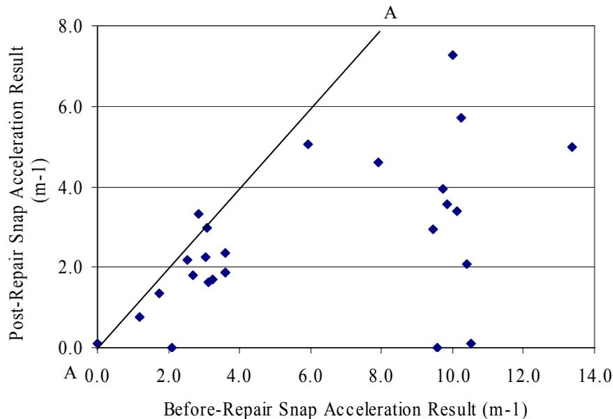
**Figure 22: After-Repair Snap Acceleration Results Versus Before-Repair Snap Acceleration Results for the 27-Vehicle Field Repair Data Set.**
