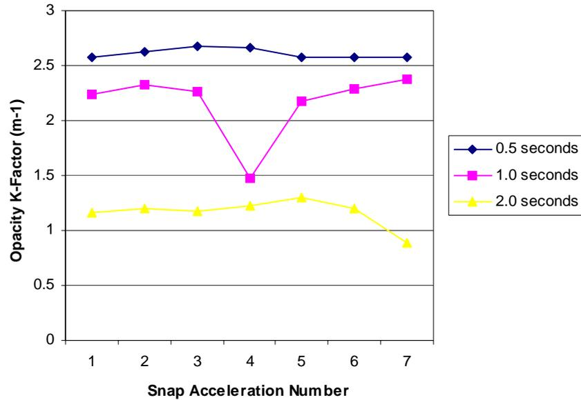
**Figure 24: Successive Snap Acceleration Results for a Mitsubishi Canter Tested at Different Rates of Accelerator Depression.**
