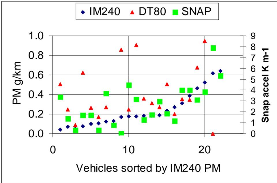
**Figure 59: PM Emissions Sorted Lowest to Highest over the IM 240 Cycle, Data for the DT 80 Cycle and Snap Acceleration also Included, for EFRU Light Vehicle Tests.**
