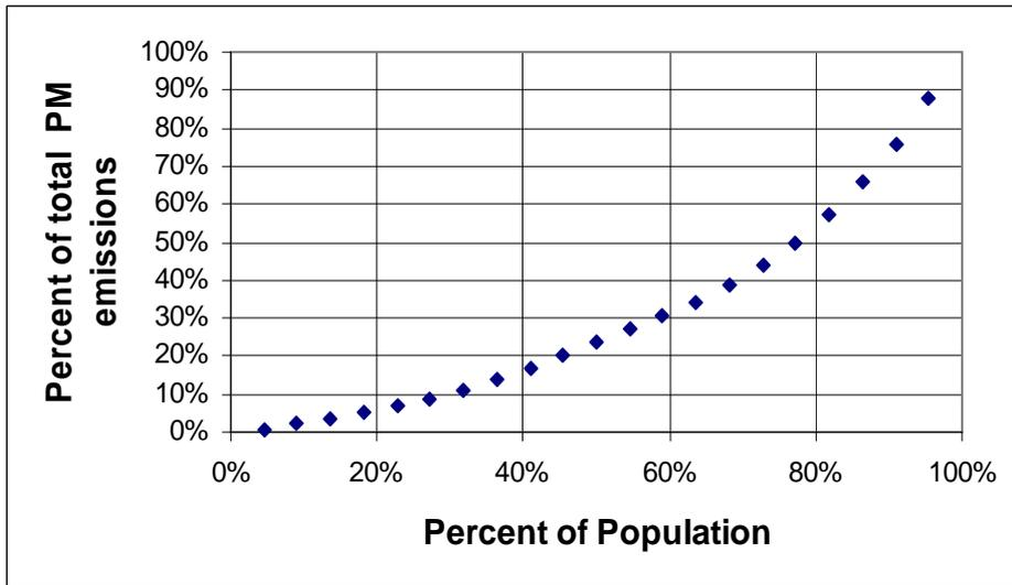
Figure 58: Percent of PM Emissions Versus Percent of Fleet Based on the IM240 Drive Cycle for EFRU Light Vehicle Tests.
