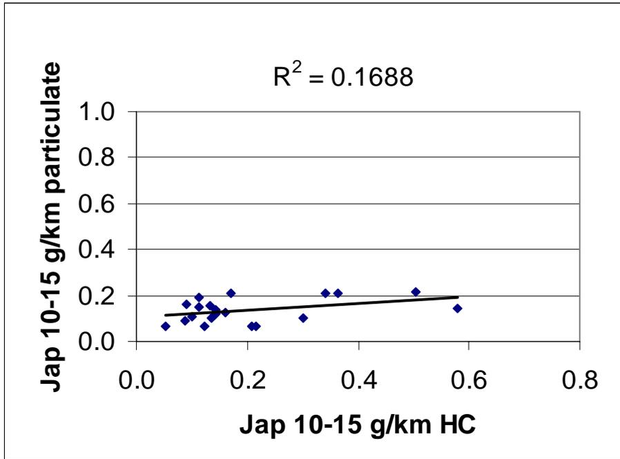
Figure 45: Jap10-15 PM (g/km) Versus Jap10-15 HC (g/km) for EFRU Light Vehicle Tests.
