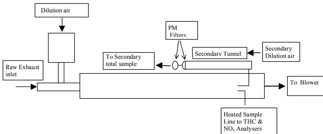
**Figure 30: Schematic of the Diesel Particulate Sampling System.**
