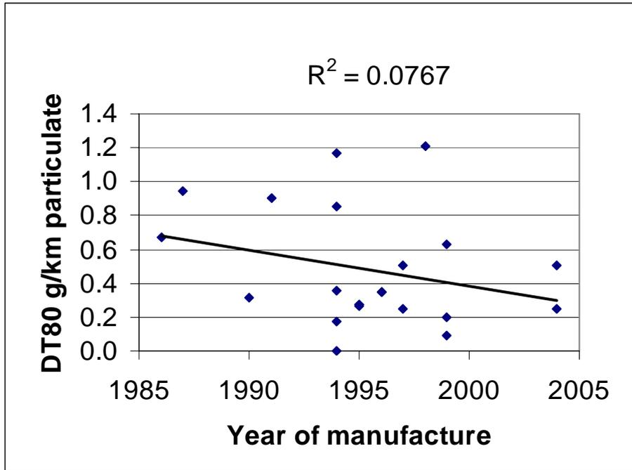
Figure 51: DT80 PM (g/km) Versus Year of Manufacture for EFRU Light Vehicle Tests.
