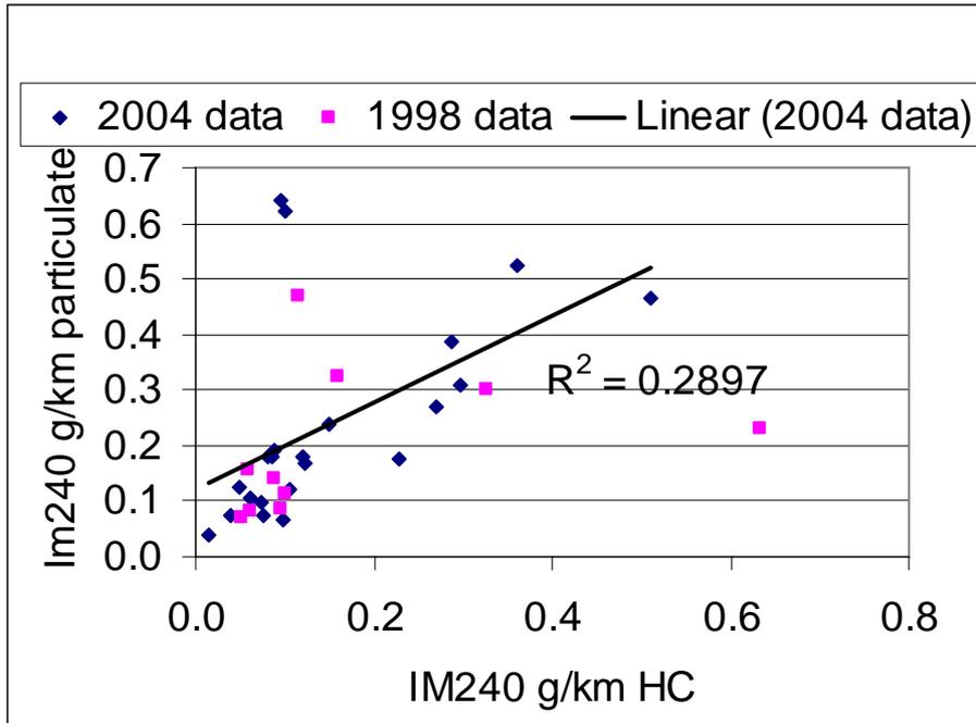
Figure 43: IM240 PM (g/km) Versus IM240 HC (g/km) for EFRU Light Vehicle Tests.
