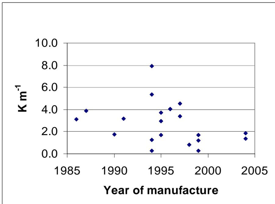
Figure 52: Snap Acceleration Results ( $K m^{-1}$ ) Versus Year of Manufacture for EFRU Light Vehicle Tests.
